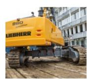
Hydraulically adjustable Undercarriage
