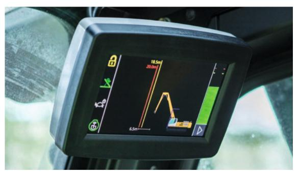
The LDC system is ergonomically arranged in the operators field of view so that it is easy and fatigueless to monitor. If a critical measure value is exceeded the LDC system au-
